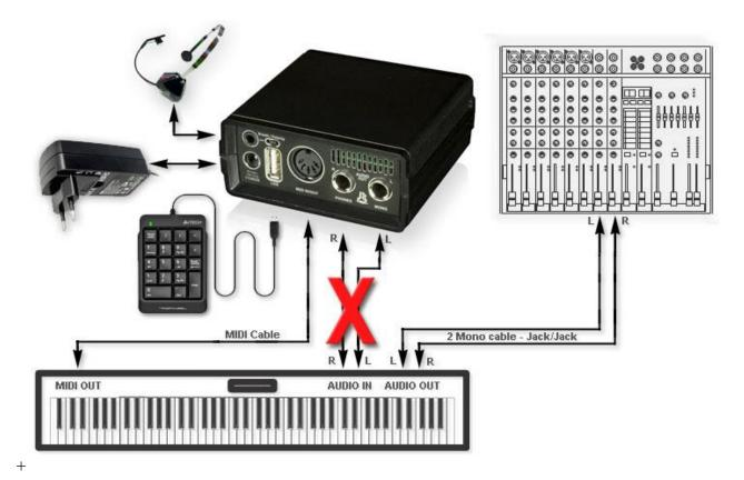
Always connect the audio output of the sampler DIRECTLY to a mixing console, not through the audio input of the synthesizer. In this picture audio connections are INCORRECT and leads to a DRASTIC reduction in sound quality. The correct way is shown in previous picture!
