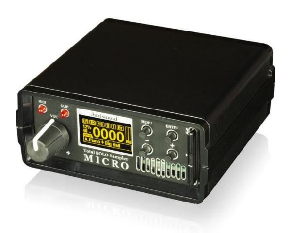
Juzisound Total SOLO Sampler MICRO, have 4 onboard buttons. With this 4 onboard buttons possible to go to every menu and set every parameter in device. Some onboard buttons have individual functions, and current button function dependent from current menu context or selected parameter. Some onboard buttons have combinations with another button. In this case is important who of both buttons are pressed first and who is second. Some onboard buttons have "long pressing" functions too.
