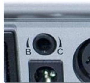
[BC] connector is on the rear end of the panel of the sampler and is used for connecting an analog controller. Analog controller means the following: controller, pedal, potentiometer or any other type of device which produces an analog signal. This connector provides power of +5 volt direct current (DC) and the input signal must also be between 0 to +5 volts. In this input most often are plugged breath controllers from Juzisound or Yamaha model BC-3.
